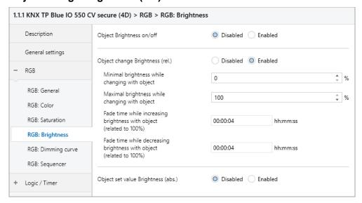
To change the brightness via relative dimming commands, there is the following object if it has been activated via parameters:
