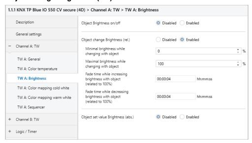
The following objects are available for changing the brightness via relative dimming commands, if they have been activated via parameters:
