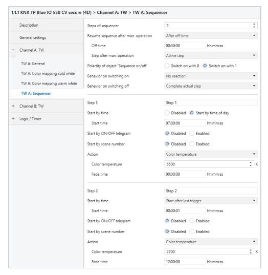
The sequencer can be used to create complex sequence programs consisting of up to 32 individual steps for the dimmer channel. The activation of the individual steps is possible at the following start conditions:
