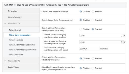
The following objects are used to control the color temperature via temperature value, if they have been activated via parameters:
