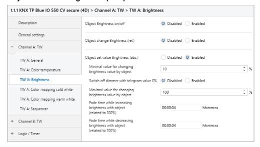
The following objects are used to control brightness via dimming value if they have been activated via parameters:
