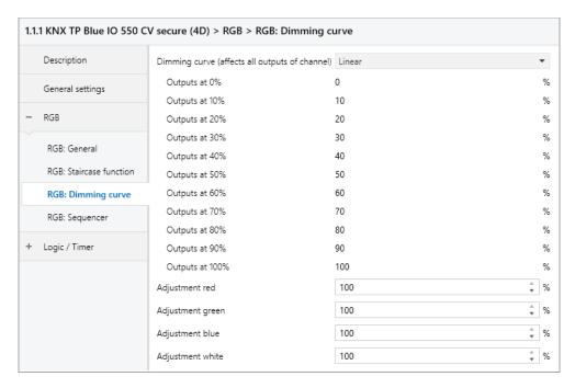
This parameter page is used for fine adjustment of the dimmer to different lamps.
