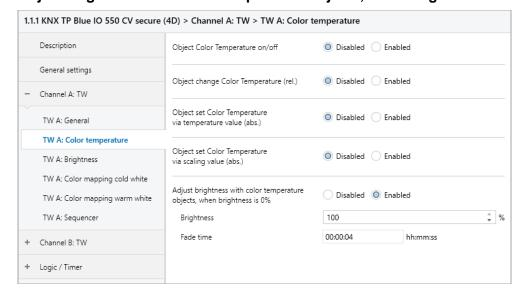
If the current brightness is 0 % and the color temperature is changed via one of the objects in the Color temperature parameter block, the brightness is dimmed to the set brightness at the same time. If the current brightness is > 0 %, this parameter has no effect on the brightness.
