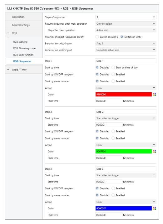
The sequencer can be used to create complex sequence programs consisting of up to 32 individual steps for the dimmer channel. The activation of the individual steps is possible at the following start conditions:
