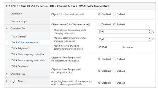
To change the color temperature via relative dimming commands, the following objects are available, if activated via parameters:
