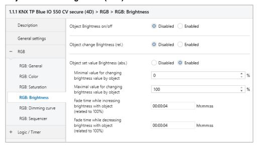
The following object is used to control the brightness via dimming value if it has been activated via parameters:
