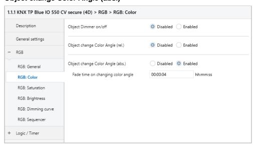
To set the absolute value of the color angle, there is the following object, if it has been activated via parameters:
