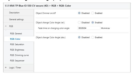
To change the color angle via relative dimming commands, there is the following object, if it has been activated via parameters:
