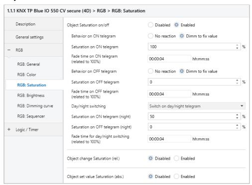
The following object is available for switching the saturation if it has been activated via parameters:
