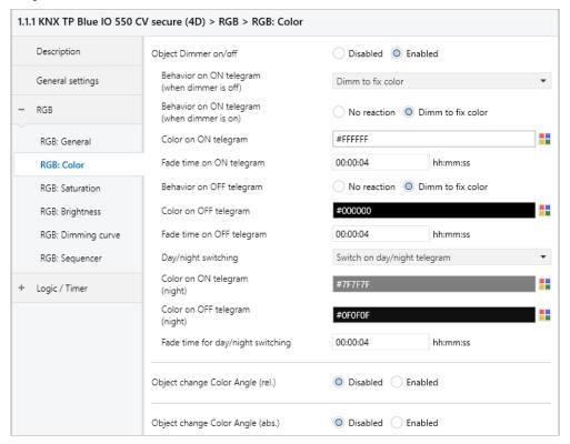
The following object is available for switching the dimmer if it has been activated via parameters:
