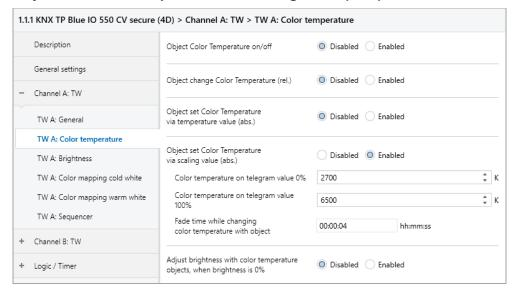
The following objects are used to control the color temperature via percentage value, if they have been activated via parameters:
