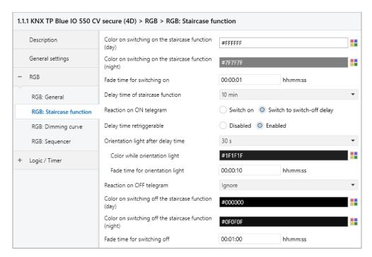
A staircase function with optional orientation light can be implemented via this parameter page. The staircase function can be overridden by the disable function. It has the following objects:
