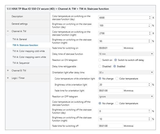
A staircase function with optional orientation light can be implemented via this parameter page. The staircase function can be overridden by the disable function. It has the following objects:
