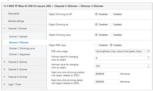
To control the dimmer via RGB color value, the following objects are available if activated via parameters:
