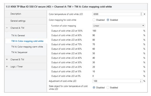
These parameter pages are used for fine adjustment of the dimmer to different lamps.
