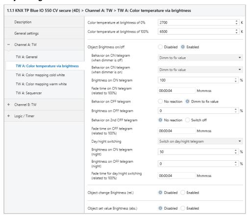
The following objects are available for switching the brightness if they have been activated via parameters:
