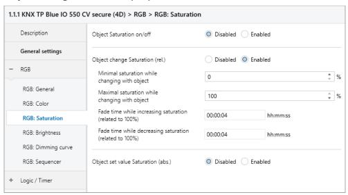
To change the saturation via relative dimming commands, there is the following object if it has been activated via parameters:
