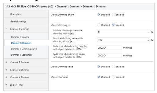
The following objects are available for dimming via relative dimming commands if they have been activated via parameters:
