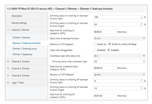
A staircase function with optional orientation light can be implemented via this parameter page. The staircase function can be overridden by the disable function. It has the following objects:
