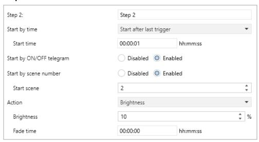
When a step is activated, its parameters appear for configuration.
