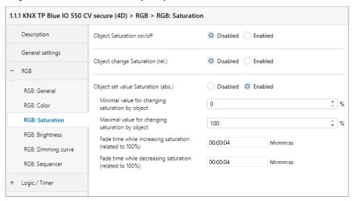
The following object is used to control saturation via dimming value if it has been activated via parameters:
