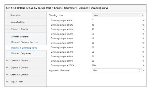
This parameter page is used for fine adjustment of the dimmer to different lamps.
