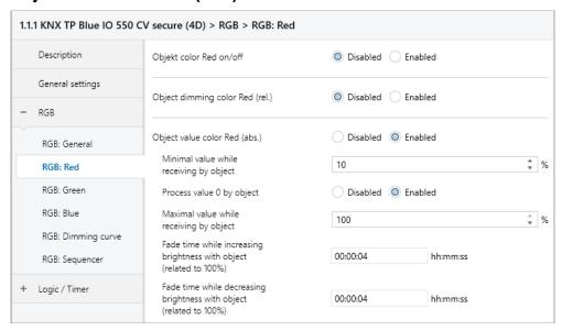
The following objects are used to control the 3 colors via dimming value, if they have been activated via parameters:
