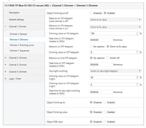
The following objects are available for switching the dimmers if they have been activated via parameters:
