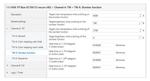
If the slumber function is selected, the following object is visible:
