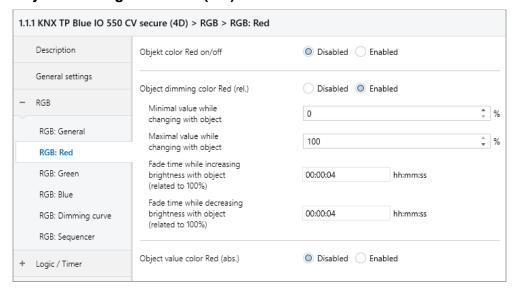
The following objects are available for dimming the 3 colors via relative dimming commands, if they have been activated via parameters:
