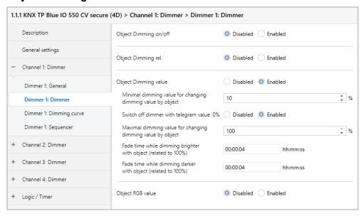
The following objects are used to control the dimmer via dimming value if they have been activated via parameters:
