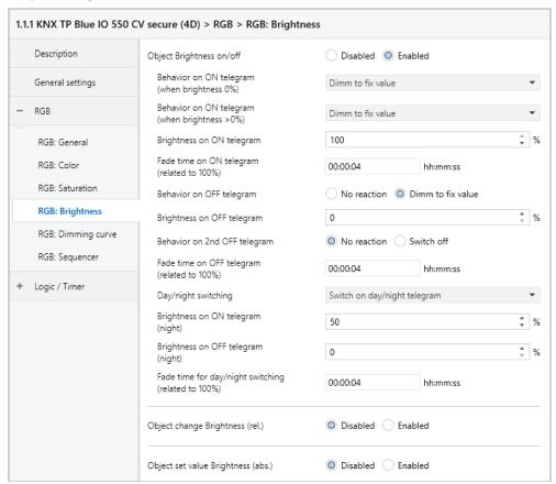
The following object is available for switching the brightness if it has been activated via parameters:
