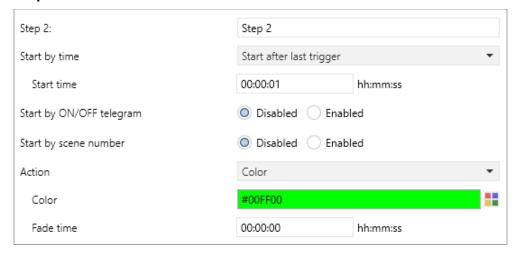
When a step is activated, its parameters appear for configuration.
