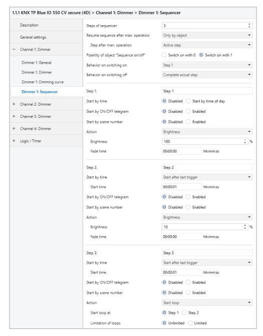
The sequencer can be used to create complex sequence programs consisting of up to 32 individual steps for the dimmer channel. The activation of the individual steps is possible at the following start conditions:
