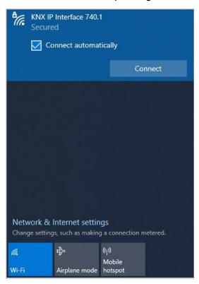
Since the KNX IP Interface 740.1 *wireless* has an integrated DHCP server, the IP address of the PC should be set automatically (DHCP). This is the default setting for most laptops.
