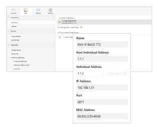
The individual KNX device address and the individual KNX addresses for additional tunneling connections can be changed within the ETS project, after the device has been added to the project.
