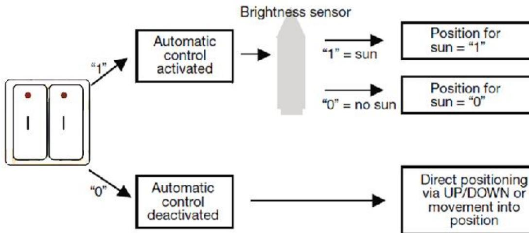
The brightness sensor is used to sense the light intensity. The push button can be connected with the universal interface or substitute for other switch sensor on the bus.
