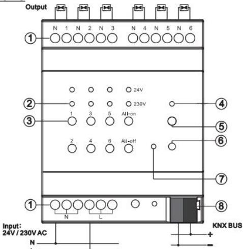
① 24V / 230V AC drive voltage input terminals, output terminals. The output terminals do not require connect to N additionally and the N are internally connected.
