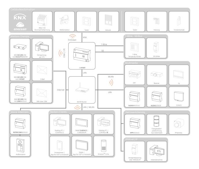
With the help of virtual group addresses (a definable KNX address range, which is only processed within the EIB**PORT**), services can be linked with each other as desired.
